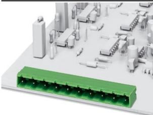
Header, nominal current: 12 A, rated voltage: 400 V, pitch: 7.5 mm, no. of positions: 12, mounting: Soldering
